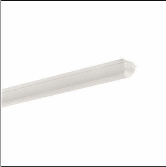
Monsun® 21 Gen.1, cover, primary optical cover: enclosure, of PC, opal, installation type: surface-mounted, LED, length: 1.571mm, width: 84mm, impact resistance: IK08, packaging unit: 1 piece
