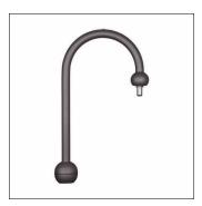
Large Bell, curved mast extension, curved mast extension, aligned, of steel, galvanised, coated, Siteco® metallic grey (DB 702S), 1-arm, with bayonet catch, diameter: 89mm, height: 1040mm, spigot size: 76/89mm (post-top), packaging unit: 1 piece
